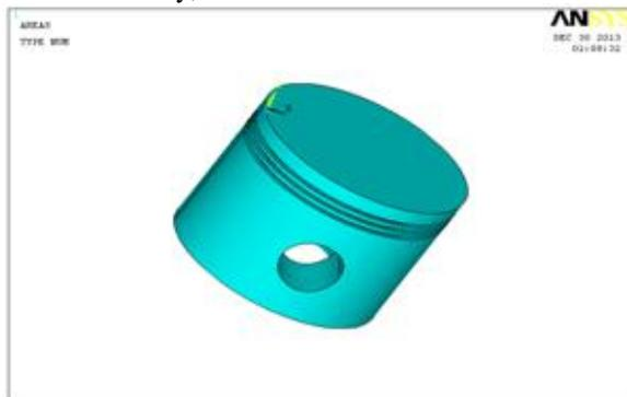
Figure 3.1 Model of Piston
